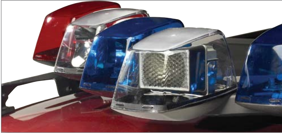
The Opticom™ emitter is available as an installed option on Federal Signal lightbars.
